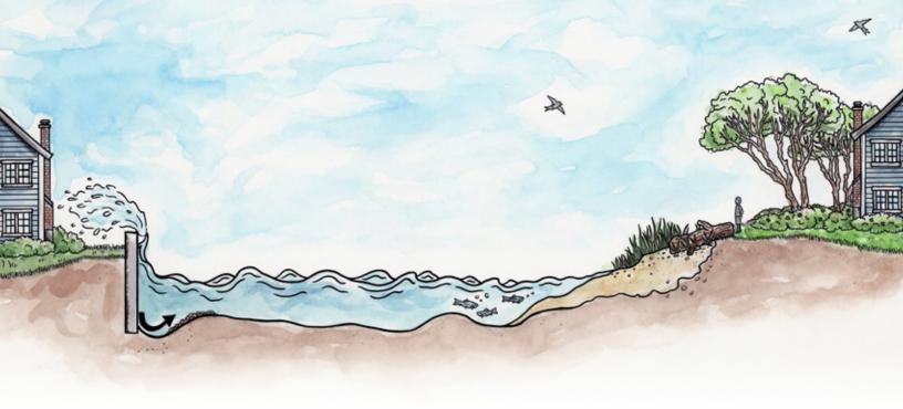
**Figure 7.2** – Coastal squeeze occurs where structures like seawalls impede the natural shoreline to adjust to rising sea levels. Natural shorelines leave room for vegetation and tidal zones to move landward.
