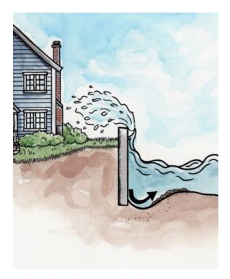
**Figure 5.1** – Impacts of shoreline modification, such as this seawall, include benthic scouring, deflected wave energy, habitat loss, and risks of flooding to the properties they are supposed to protect.
