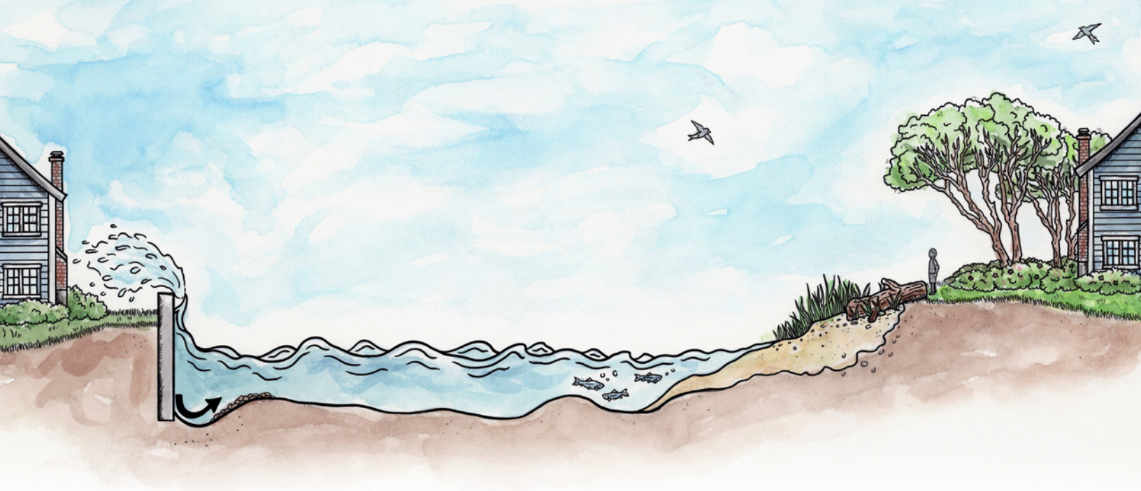
Figure 7.2 – Coastal squeeze occurs where structures like seawalls impede the natural shoreline to adjust to rising sea levels. Natural shorelines leave room for vegetation and tidal zones to move landward.
