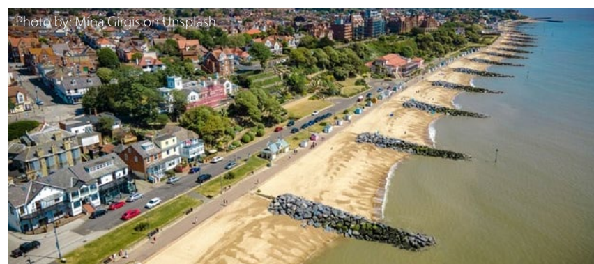
Figure 10 – Coastal squeeze occurs where structures like seawalls impede the natural shoreline to adjust to rising sea levels.
