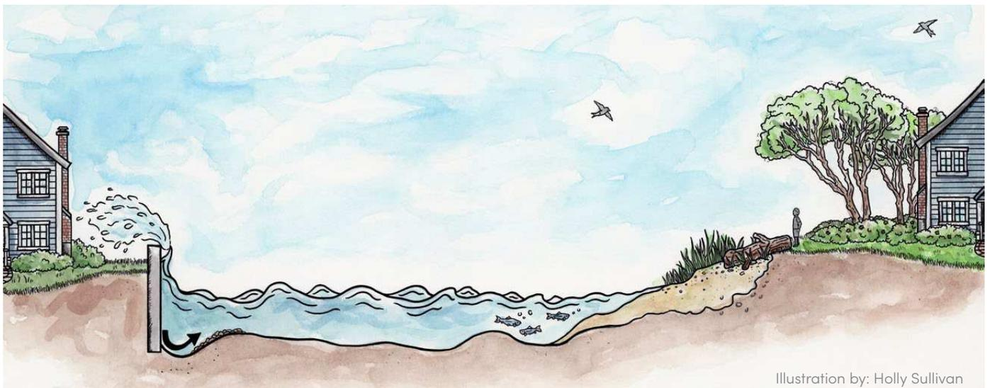
**Figure 2.** Coastal Squeeze occurs where structures like seawalls impede the natural shoreline from adjusting to rising sea levels. The left side of this illustration depicts a seawall in place of habitat which has been lost due to rising sea levels, erosion and scouring. On the right side, a natural shoreline leaves room for vegetation and tidal zones to move landward, preserving important habitats and their function.
